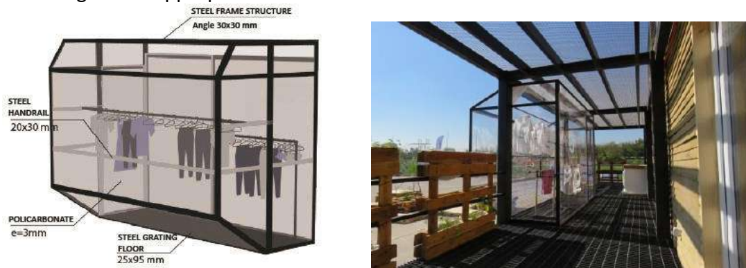
Figure 8. Solar clothes dryer design. Figure 9. Team photo: solar clothes dryer integrated in the prototypes terrace.
