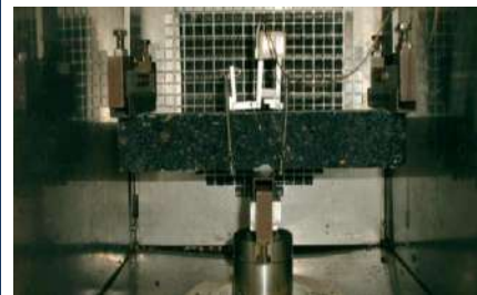
Three-point bending test (3PB) Annex C
